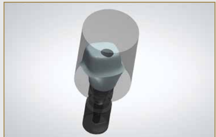
Figure 8: The milling blank slider should be used to verify that the design can be contained within the dimensions of the millable area.
