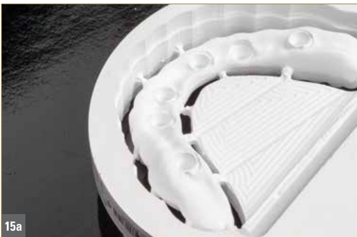
Figures 15a, 15b: Following milling, the prosthesis is removed from the BruxZir™ blank (Glidewell Laboratories; Newport Beach, Calif.), with the support structure left in place so the appliance can remain upright during sintering.
