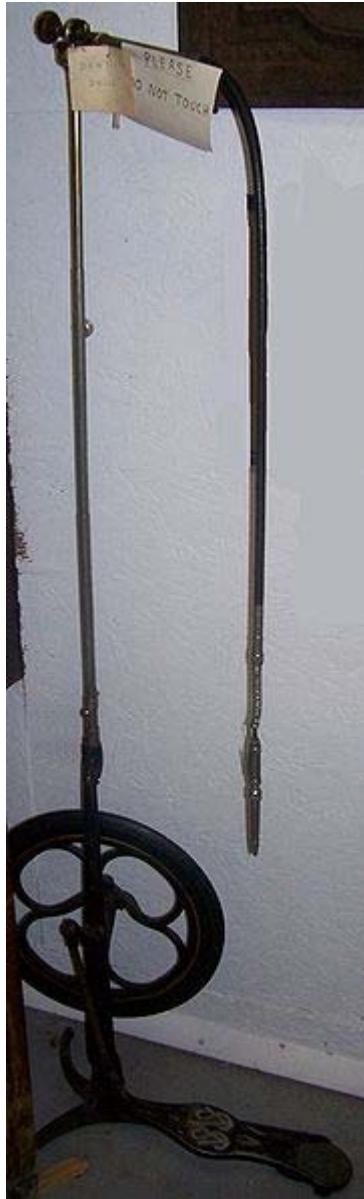
Foot-powered dental drill
