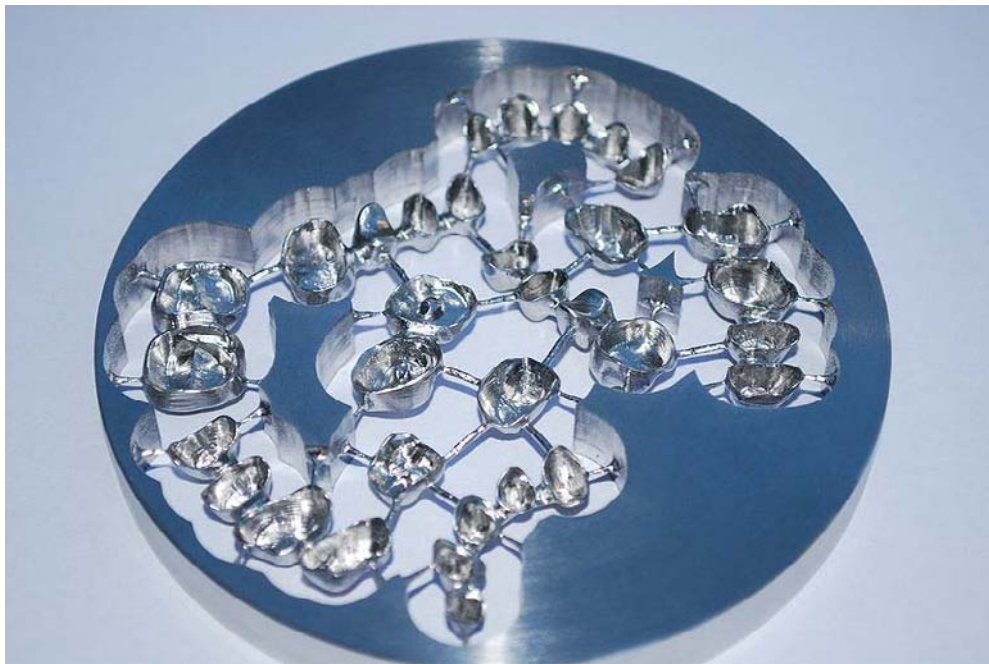
Chrome-cobalt disc with bridges and crowns for dental implants manufactured using WorkNC Dental CAD/CAM
