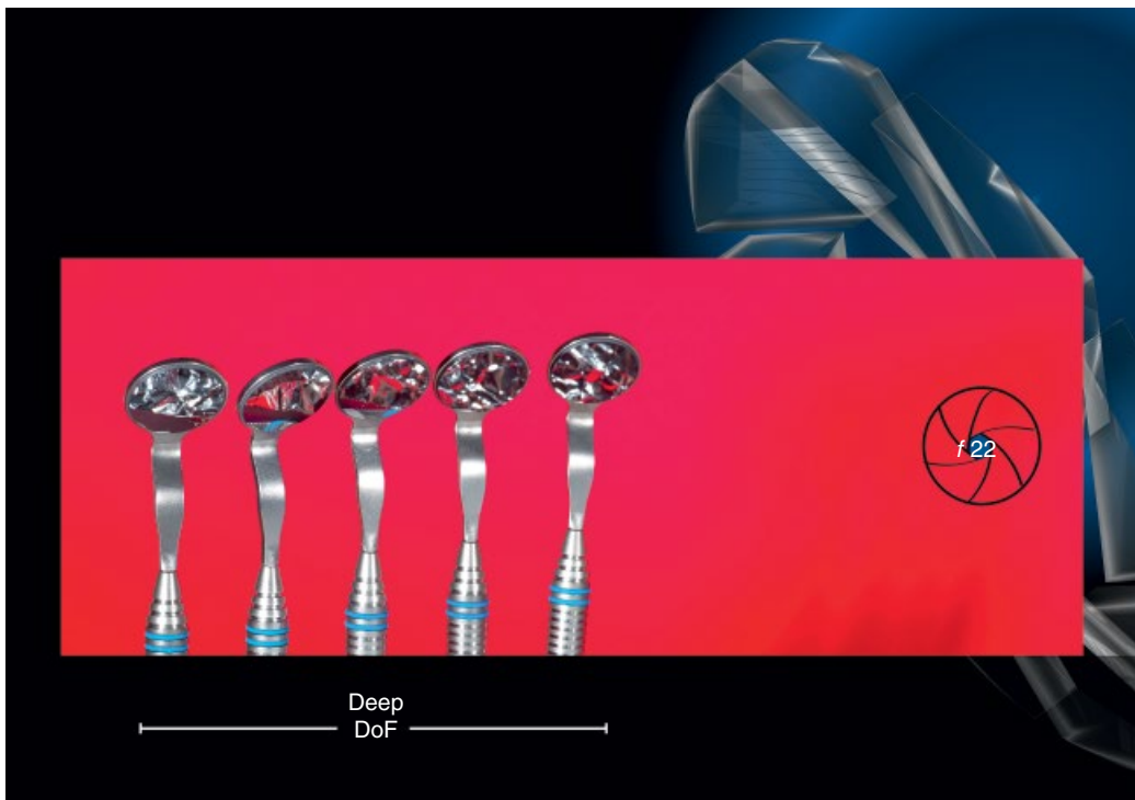
Figure 3.15 Deep depth of field (DoF): small aperture (large f number), all five mirrors are sharply focused.
