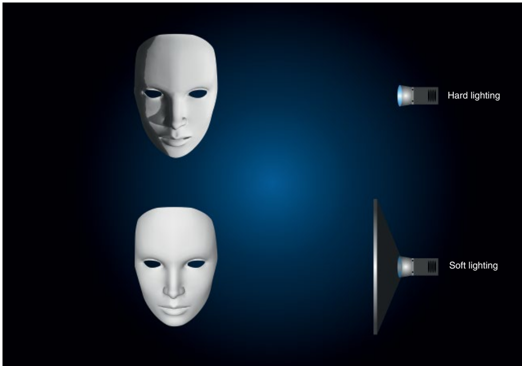
Figure 6.19 A hard light, produced by a naked light source, emphasises facial features (notice the shadows on the right side of the face contralateral to the light source), whilst soft light attenuated by diffusers, such as soft boxes, tends to smooth out detail.
