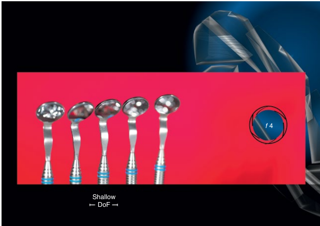
Figure 3.14 Shallow depth of field (DoF): large aperture (small f number), only the third mirror from the left is in sharp focus.
