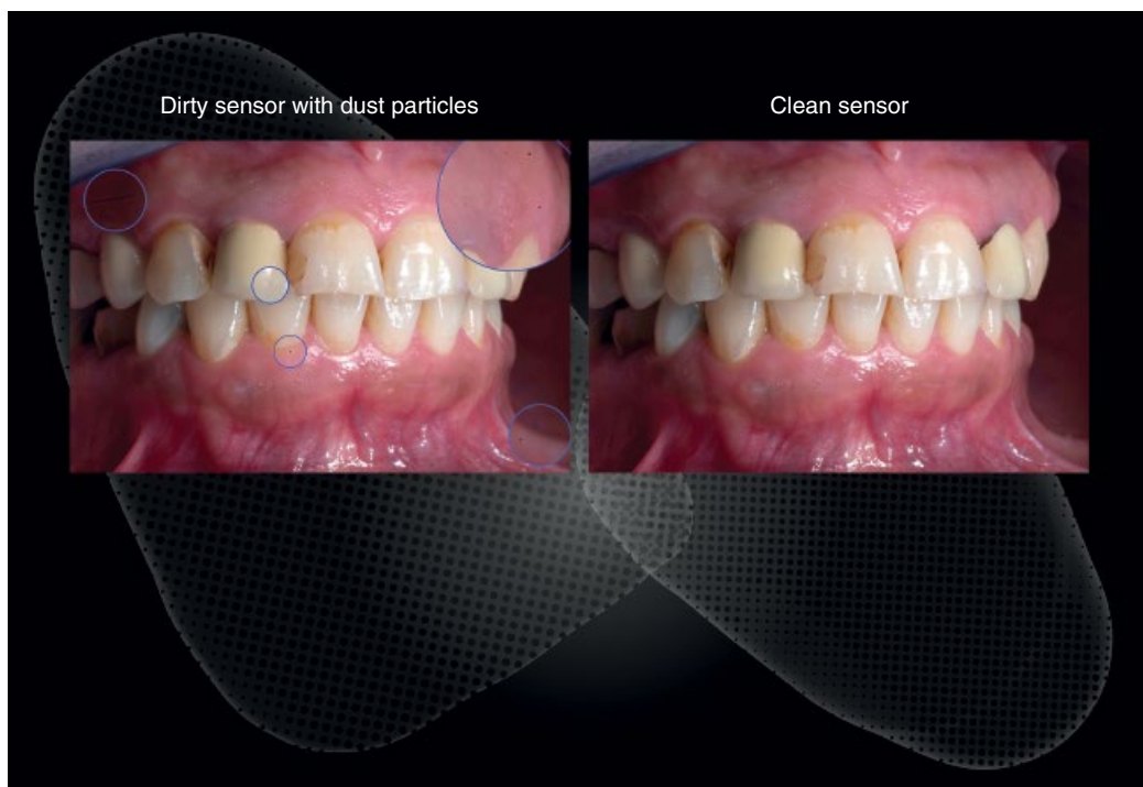
Figure 1.13 Dust particles adhering to the sensor surface are particularly conspicuous against light-coloured backgrounds.
