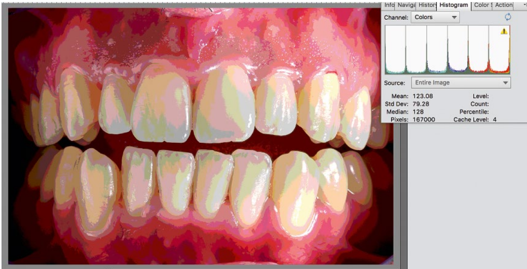
Figure 9.7 Posterisation: colour histogram showing a spiky appearance representing colour banding without seamless transition between missing colours.
