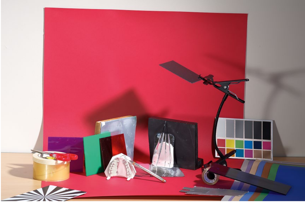
Figure 7.20 Improvised set-up for bench images, consisting of various coloured backgrounds, reflectors, mirror, Perspex sheets, clamps, grey card, etc., which can be tailored as necessary for a specific photograph.
