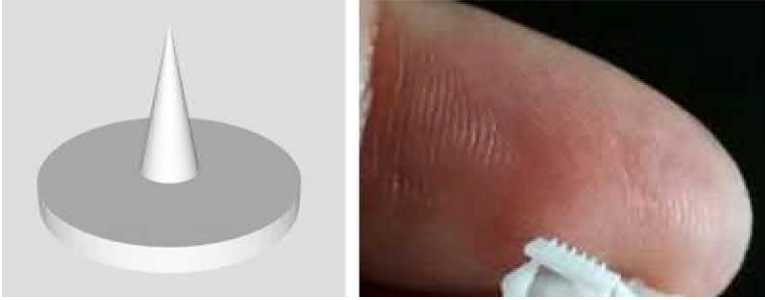
FIGURE 54.8 SLA printed high-resolution microneedles.
