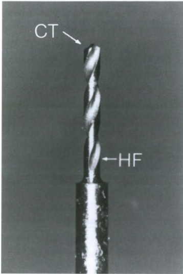
Fig.3-13 A closeup view of a 0.6-mm-diameter twist drill shows the cutting tip ( CT ) and helical flutes ( HF ).
