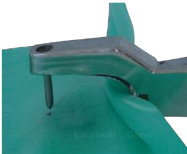
Fig. 6. An hole position felt-tip marked by the template eases the piercing of the sheet in the right position.
