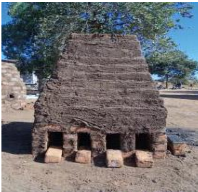
Side view of brick kiln showing air inlets at the base
