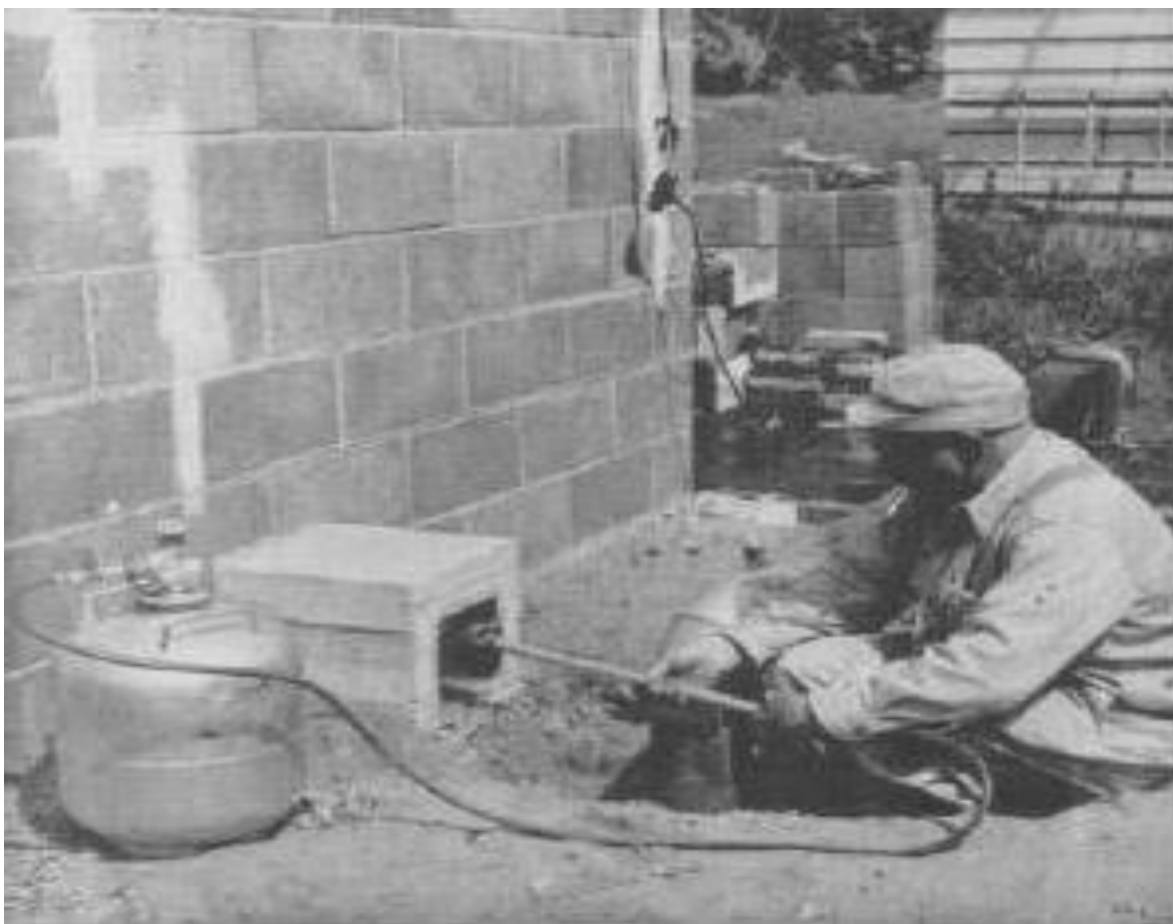
Igniting the kiln charge with a torch.
