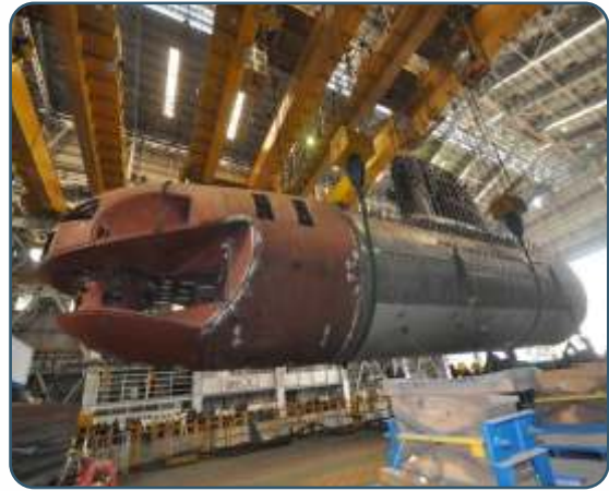
Lifting of joined sections
