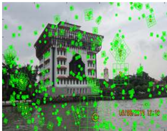
Fig 13. Step 2 of SIFT algorithm- description of Key-points
