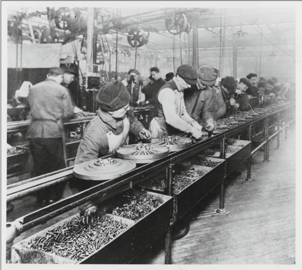
Workers on the first moving assembly line put together magnetos and flywheels for 1913 Ford autos. By an unknown photographer, Highland Park, Michigan, 1913.
